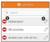
Touch the remove icon (as shown at 1 in the image) next to the name of the plan you would like to remove.
