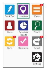
Working with Locations on EnSURE Touch is effortless! Locations are test points, from which you take a sample for testing.
