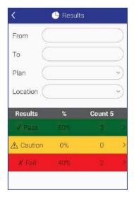
The Results screen will display all the results currently on your unit. You are able to filter by date, plan, and location. The table area below the filters will display a total count of all Pass, Caution, and Fail results based on the filters selected above.
