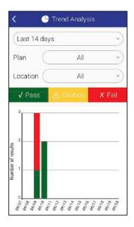
The Trend Analysis screen displays a breakdown of your total results in an easy to view graph that separates Pass, Caution, and Fails. You can filter the results by date, plan, and location.
