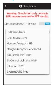
Turning on Simulation Mode converts the RLU results from ATP testing on your EnSURE Touch so that they simulate the results you'd get if you were using another system.
