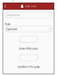
Enter a **Username** for the new user and then select a **Role**. Users can be setup up as Operators or Administrators. Operators perform testing while Administrators manage the instrument and have access to all of the settings.
