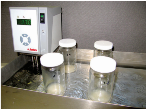
Figure 4. Picture showing a 2mag Mixdrive 15 ® submersible magnetic stirrer in a custom made water bath. This allows stirring of 15 samples at controlled speed (170 rpm) and 37°C.
