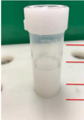
**Wet sample** (0.5 g) with 0.5 mL of ethanol and incubate in 20 mL of **sodium maleate buffer** (50 mM, pH 6.0) containing 2 mM  $\text{CaCl}_2$  at 37°C with **2 KU PAA** and **0.85 KU AMG** and stir at 170 rpm.
