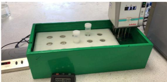
**Figure 2. Incubation Method 1.** Samples (~ 0.5 g) in 40 mL, 30 x 84 mm polypropylene tubes in a designed polypropylene tube holder (Megazyme cat. no. **D-PPSTH**) [ $C(w)$ ] on a 2mag Mixdrive 15<sup>®</sup> submersible magnetic stirrer in a custom made water bath (Megazyme cat. no. **D-TDFBTH**). This arrangement allows stirring of 15 samples at controlled speed (170 rpm) and 37°C.
