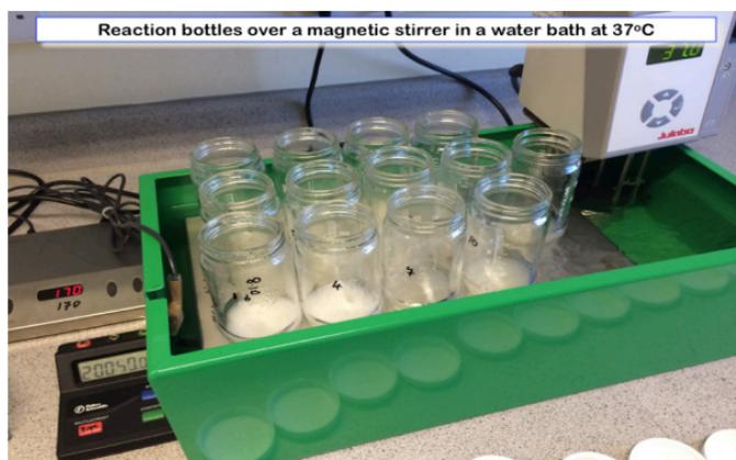
**Figure 3. Incubation Method 2.** Samples (~ 1.0 g) in Fisherbrand bottles on a 2mag Mixdrive 15<sup>®</sup> submersible magnetic stirrer in a custom made water bath (Megazyme cat. no. **D-TDFBTH**). This arrangement allows stirring of 15 samples at controlled speed (170 rpm) and 37°C.
