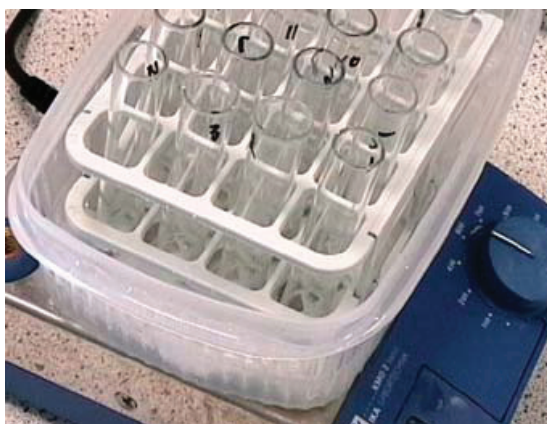
Figure 2. Arrangement of ice-water bath over a magnetic stirrer for treatment of samples with 2 M KOH and dissolution of RS.
