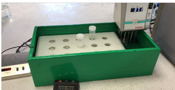
Figure 2. Incubation Method I. Samples (~ 0.5 g) in 20 mL of buffer plus enzymes in 30 x 84 mm polypropylene tubes in a designed polypropylene tube holder (Megazyme cat. no. D-PPTH) on a 2mag Mixdrive 15 ® submersible magnetic stirrer in a custom made water bath (Megazyme cat. no. D-TDFBTH ). This arrangement allows stirring of 15 samples at controlled speed (170 rpm) and 37°C.
